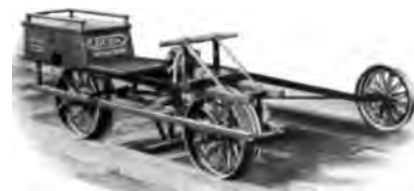
Buda No. 10-NH. Motor Velocipede Car
